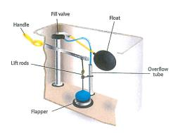
Another simple test is to turn off the toilet inlet water valve on the wall. Mark the level of the water on the inside of the tank. If the water level drops in one hour, it is leaking.
